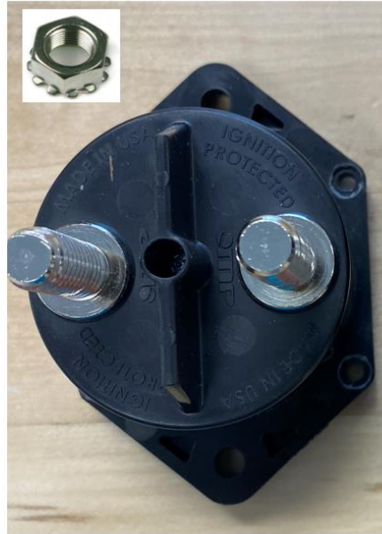
Rear view: Bussmann and Blue Sea Systems Series 187 (left) with offset studs and special nut hardware vs. MP Series 87 (right) with center-positioned studs and standard Sems nut (inset).
